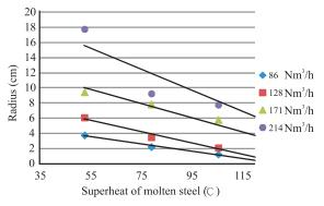
Fig.7. Relationship between mushroom radii and the molten steel temperature under different gas flow rates.
