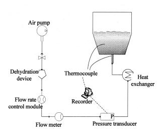
**Fig.1.** Schematic illustration of the water model with its gas supply system.
